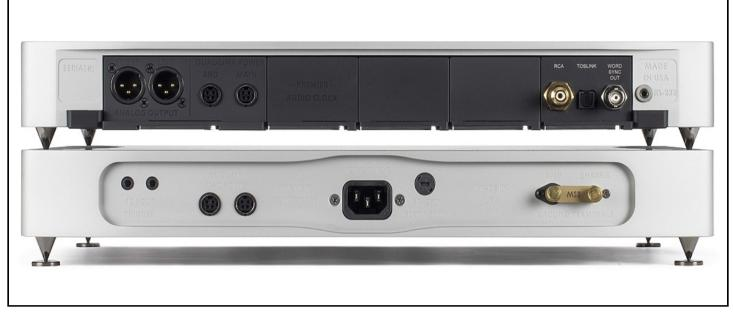
In its basic form, the Powerbase provides isolated power for the DAC circuits only. However, its operation can be boosted by providing enhanced grounding to an amplifier via a supplied cable. Once again, this constitutes neatly thought-out and rather useful added functionality from MSB Technology. Once experienced, there is no going back, so I contentedly used the Powerbase throughout the review period.
